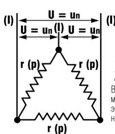
Watt density (W/cm<sup>2</sup>) for each element is unchanged
