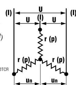
Watt density (W/cm<sup>2</sup>) for each element is unchanged
